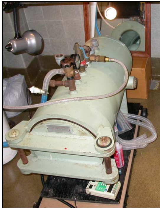
Figure 4: Hyperbaric oxygen chamber specially designed for animal research. Rear end glass window permits animal monitoring using the mirror behind the chamber.
